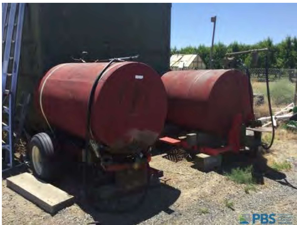
Photo 40. Mobile ast gasoline tanks.
