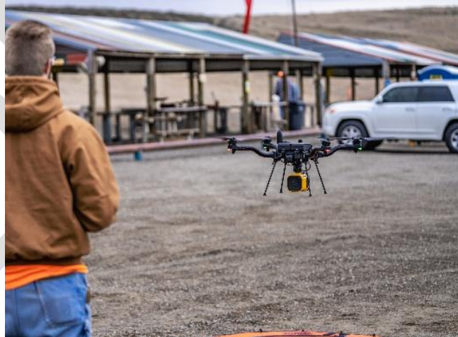
RSI's unmanned autonomous vehicle in takeoff with LiDAR mapping unit payload.
