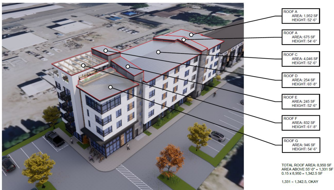
Figure 4 – Roof Plane Analysis
