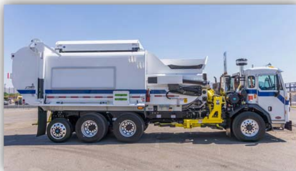
FIGURE 3.1: SCORPION ASL BODY WITH CNG TANKS
