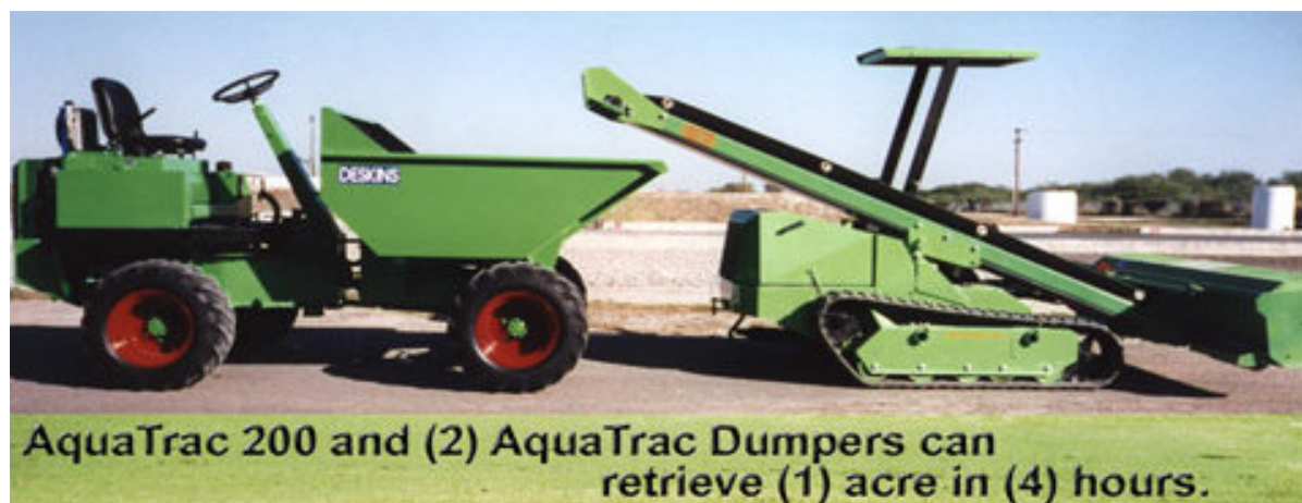
FIGURE 5 Typical Deskins Filter Solids Collection Tractor System
