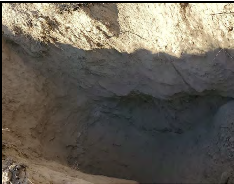
Subsurface soil profile within test pit TP-5
