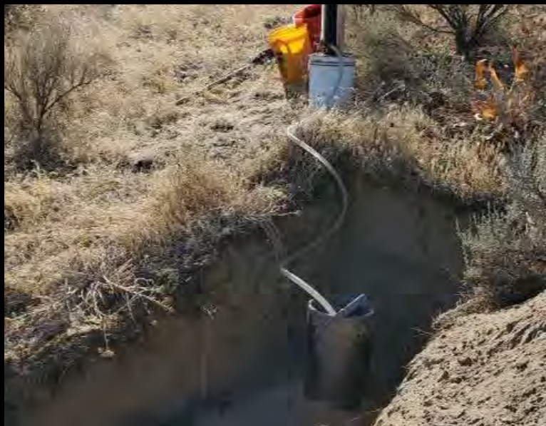
Infiltration test setup at IT-3
