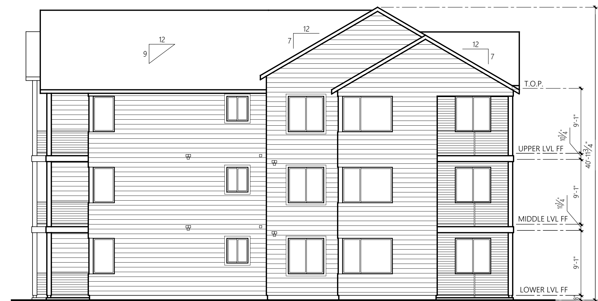
BLDG TYPE I SIDE ELEVATION 1/8" = 1'-0" Buildings 1, 3, 5, 6 & 7
