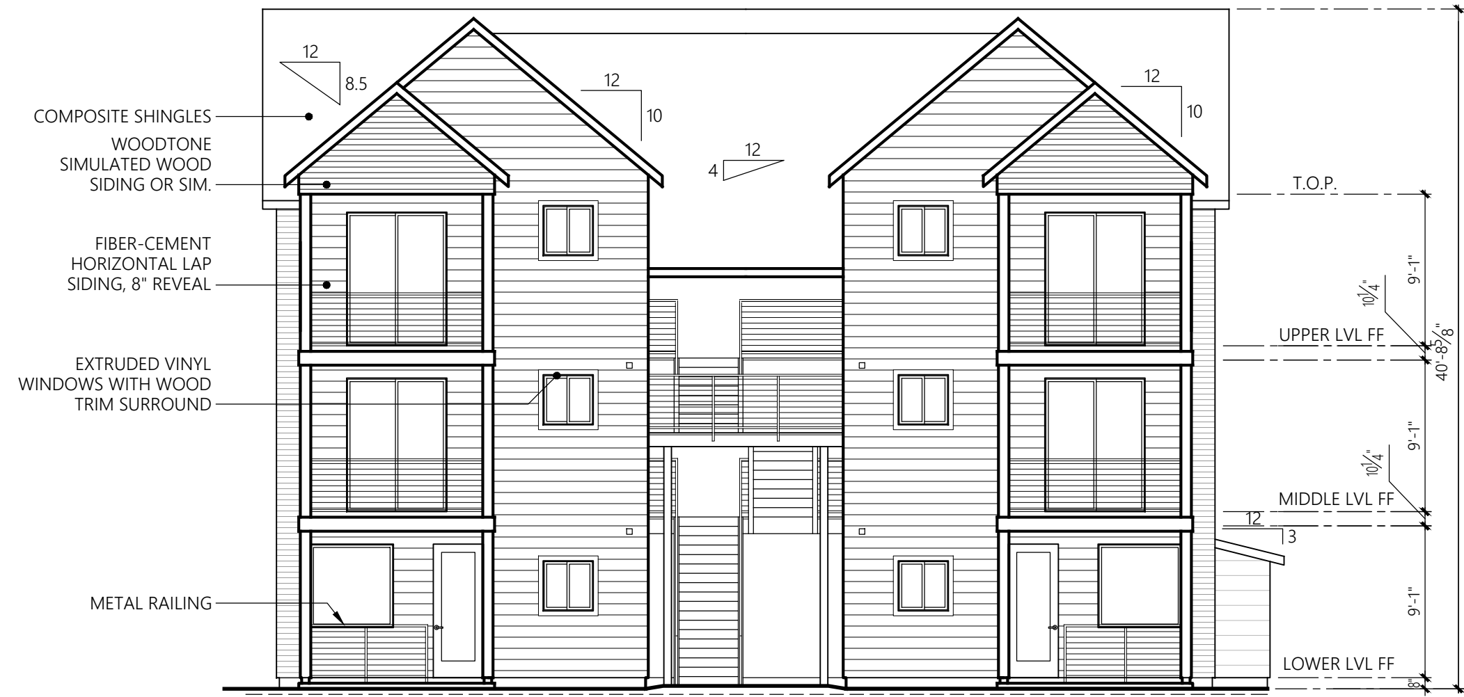
Building 4 PARKING AISLE ELEVATION 1/8" = 1'-0" Buildings 2 & 4
