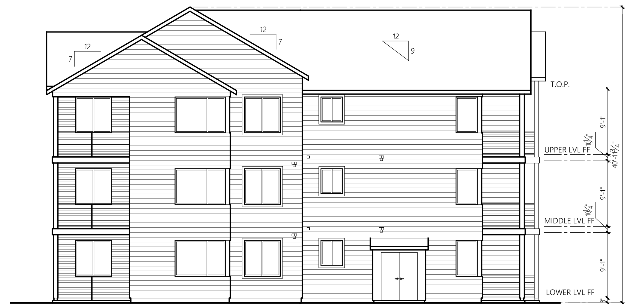
BLDG TYPE I SIDE ELEVATION 1/8" = 1'-0" Buildings 1, 3, 5, 6 & 7
